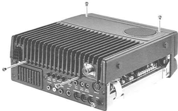
Figure 4: Top Cover/Heatsink Removal
